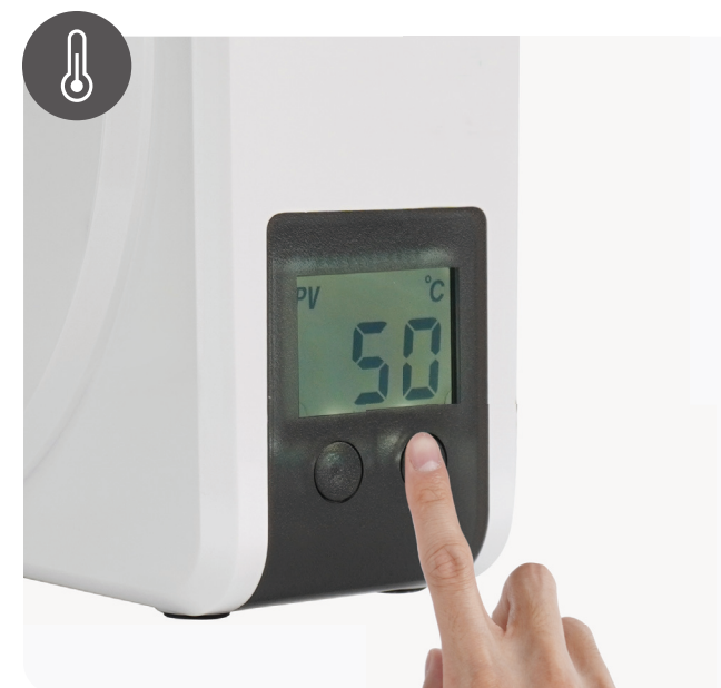
Fig4: Press Left/Right button to power on. After power-on, press Left/Right to set target temperature (35°C-55°C). Press both buttons simultaneously to power off.
